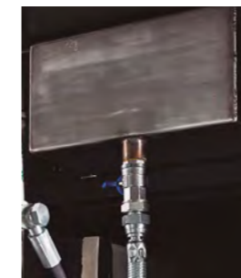
Automatic oil refill reservoir
