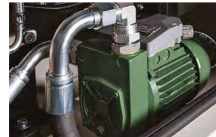
Fuel transfer pump
