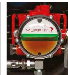
Oil level monitoring system
